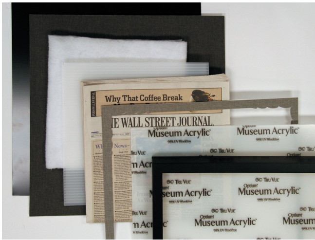
● The DCO stack of materials includes (from bottom to top): aluminum composite material reinforcement, frame-sized background of matboard, needle-punched polyester batting, Coroplast mounting board, newspaper, decorative linen mat, acrylic, 1 ¼" deep frame.
