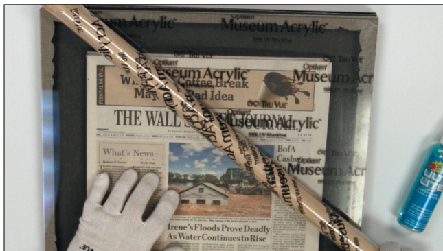
● Remove the masking from the acrylic glazing just before final assembly.
